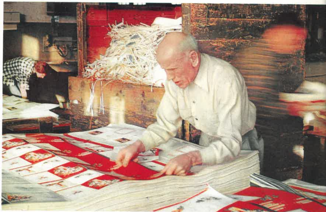
Cut-out cards are stacked for removal of waste edges.
