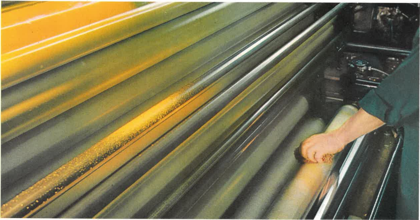
Rollers evenly distribute ink and moisture on the plate.
