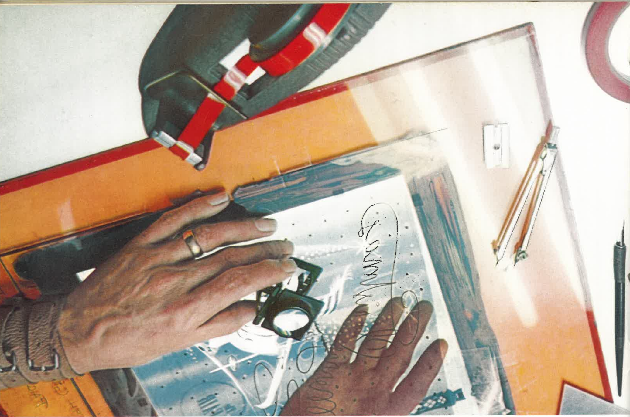
Forms are checked for close register in over-printing.
